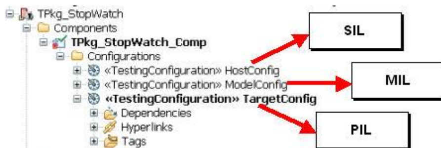
Figure 15: Different code generation configurations (MiL, SiL, and PiL)
